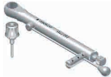
**Important:** The abutment must be positioned in the octagon before the screw is tightened. The basal screw in the RN synOcta® gold abutment is tightened to a torque of 35 Ncm.
