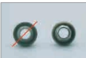
9. Carefully devest the casting using only ultrasound, water jet or pickling. **Do not sandblast!**
